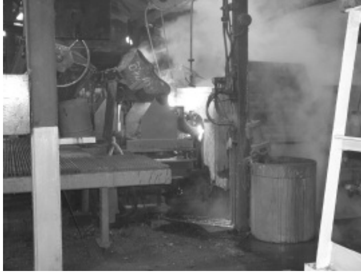
Figure 7—Iron being poured into spinning pipe mold.
